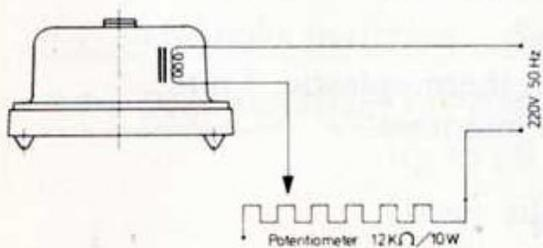
Fig. 4 Adjustment of output with potentiometer.
