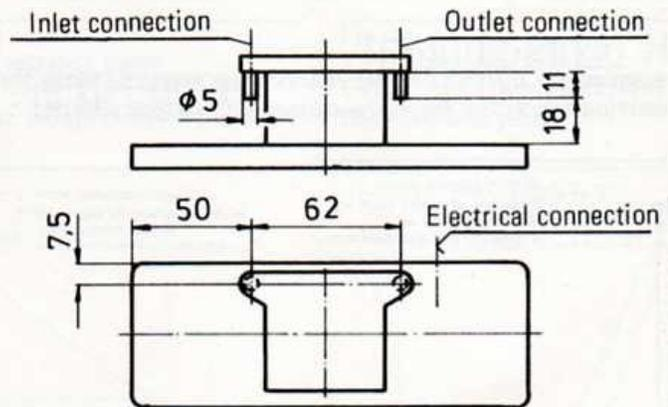
Vacuum pump, typ for installation
